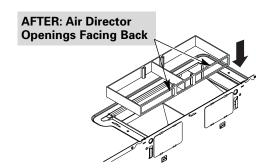
**5** Replace blower plate with the screw removed in Step 1. Make sure the screw is tight.
