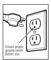
The power cord of this appliance is equipped with a three-prong (grounding) plug which mates with a standard three-prong (grounding) wall receptacle to minimize the possibility of electric shock hazard from this appliance.
