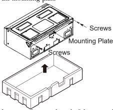
Remove the screws from each end of the mounting plate. This plate will be used as the rear wall template and for mounting. Reinstall the screws into the holes where they were removed.
