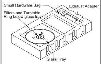
**2** Fold back all 4 carton flaps fully against carton sides. Then carefully roll the oven and carton over onto the top side. The oven should be resting in the Styrofoam.
