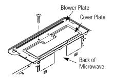
• The cover plate is installed with the blower plate, not need to unintall.
