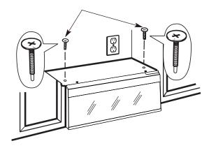
**6** Tighten the outer two screws to the top of the microwave oven. (While tightening screws, hold the microwave oven in place against the wall and the top cabinet.)
