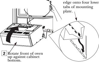
Insert a self-aligning screw through top center cabinet hole. Temporarily secure the oven by turning the screw at least **two full turns**fter the threads have engaged. (It will be completely tightened later.) Be sure to keep power cord tight. Be careful not to pinch the cord, especially when mounting flush to bottom of cabinet.
